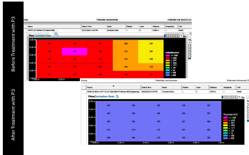
Figure 4: Field QC Results, Half-Cell Corrosion Potential Testing, Parking Garage, UAE 2024
