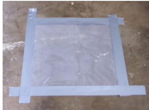
Figure 1: Plastic test square (from constructor.org)
