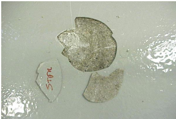
Figure 1: Debonded Epoxy (Lawrence)
